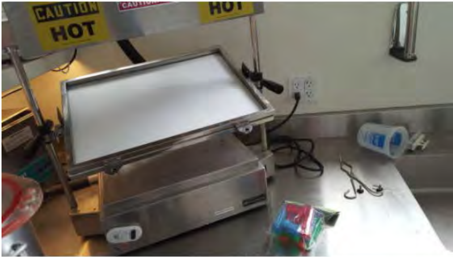
The vacuum forming process is paired up with the reality 3D capturing and scanning process. The initial attempt was to 3D scan the guns, then 3D print a mold, to then mold the pieces after remodeling the piece in 3D CAD software. The vacuum form is effectively easy to use, but one should take caution when operating the machine, as it could be hot, and testing on various sacrificial water pistols are suggested.
